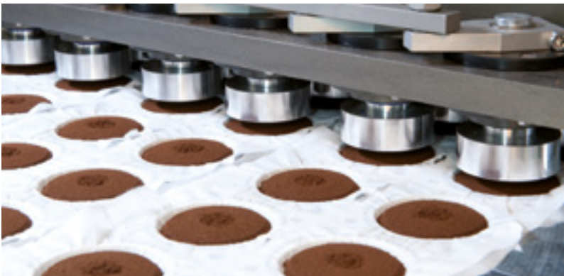
OPTIMA consumer manufactures the fastest packaging machines for coffee capsules and soft pads including highest accuracy in filling.
