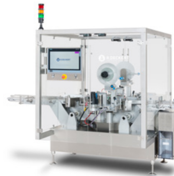
Implementation of the EU falsification guideline with folding carton labeling and TRACK & TRACE STATION.
