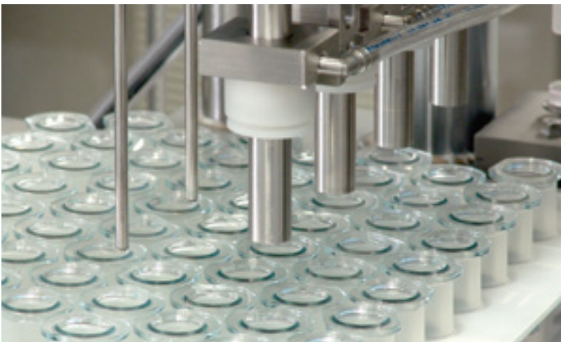
Filling machines for disposable syringes. Further containers like carpules and vials can be processed by this flexible plant.
