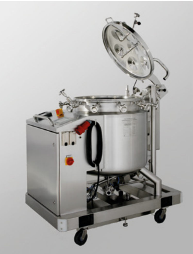
For a wide range of purposes: fermenters, bio-reactors, stirring unit and processing containers, pressure and collection containers.
